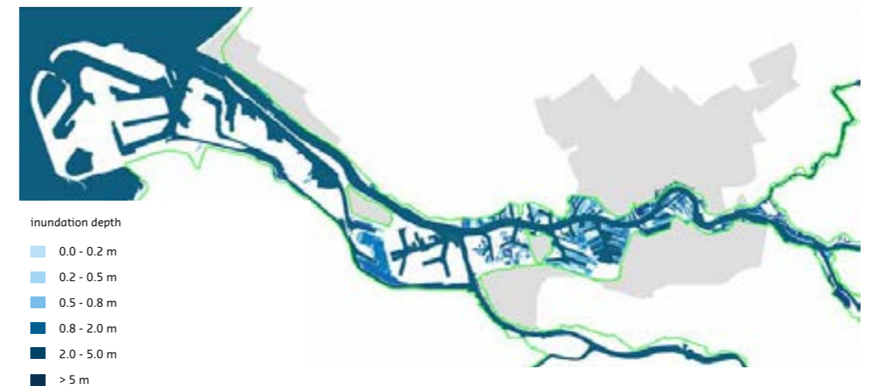
Map 2: Outer-dike flooding in Rotterdam in 2100 (source: Deltares) W+ climate scenario with a frequency of 1 x 1,000 years
